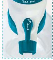
Reagent loss during ventilation is avoided with the recirculation valve.
