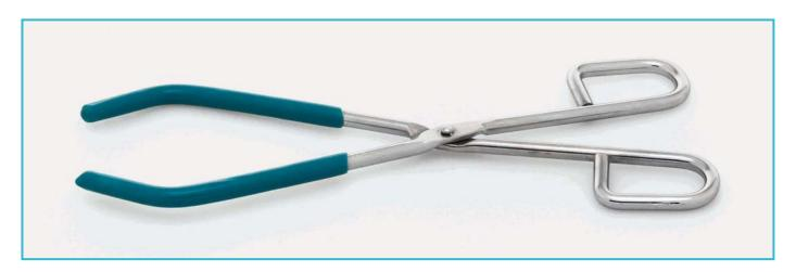
Manufactured from chromated steel. Insulated jaws are covered with special coating with perfect insulation enabling to hold all types of vessels in most secure way.
