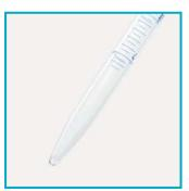
All pipettes have colour coded suction stems to allow fast identification and sorting.
